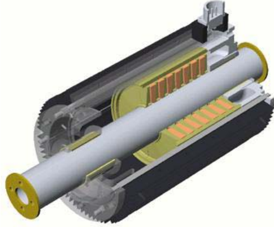
Fig. 1.2. Tubular PM LSM. Moving rod (reaction rail) contains circular PMs [192]
